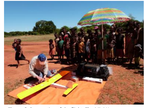
Figure 3. Preparation of the flight: The Mini Horus was equipped with two cameras (RGB), batteries and connected to the autopilot.
