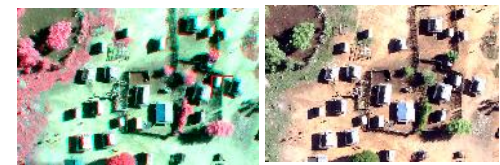
Figure 4. Aerial photograph showing the center of a village. The Mini Horus was equipped with two cameras (RGB = Casio Exilim EX-S12; IR = Fuji Finepix F30, NIR-blocking filter removed, IR-Filter 720 nm) resulting in NIR (left) and true colour (right) images.
