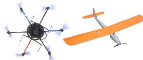
Figure 2. Hexakopter (left) and Mini-Horus (right; Breadth: 1,74 m; length: 1,25 m; weight with payload: 2,07 kg).
